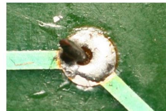
Too Little Solder
